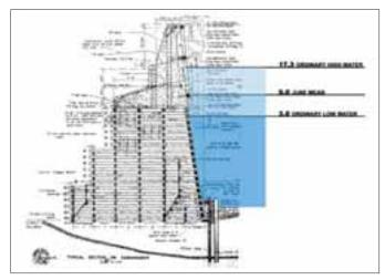
A cross-section construction drawing of the seawall, illustrating the magnitude of the structure, much of it below water.
