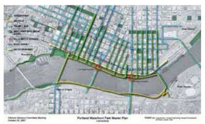
Diagram of the current circulation routes and access points to the park. The red lines indicate the many barriers or lack of formal crosswalks into the park.
